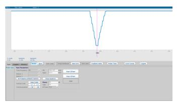
7. The default number of points is set to 512. This produces a roughly shaped tuning dip that is responsive to changes made with the match and tune knobs. You can increase the # Points from the drop-down menu to get a smoother line. This will take longer for changes to be reflected on the screen and should only be considered for fine adjustments (when the dip is already near minimum and centered).
