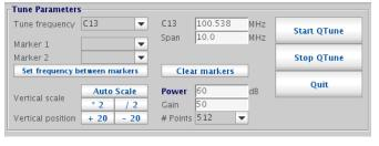
4. Click the **Start QTune** button to start the tuning process. The canvas will appear as shown here and the **Quit** button will be disabled. The LCD display on the tuning panel (where the cable is attached) will turn on, but the displayed numbers can be ignored as they don't correspond to tuning performance in this mode.
