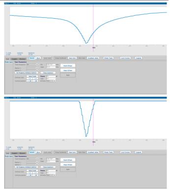
6. Use the tune (top) knob on the tuning stick of the appropriate channel on the probe to center the tuning dip about the magenta line. If needed, use the match (bottom) knob of the tuning stick to lower the tuning dip to its minimum. You may need to alternate between tuning and matching to achieve both a low and centered dip.
