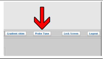
3. By default, the panel will open to H1 tuning with a blank canvas. Use the Tune frequency drop down menu to change the nucleus if tuning a different channel, such as C13.
