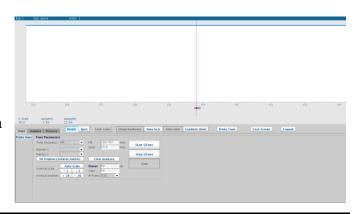
5. Click the Auto Scale button in the lower left to display the tuning dip. You can use the \*2 and /2 buttons or the mouse scroll wheel to further adjust the vertical scale and appearance of the tuning dip.
