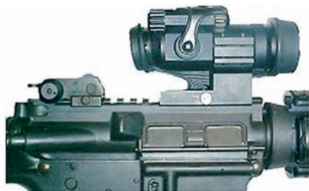
Figure 2.5 M68 Close Combat Optic Mounted on M16A4/M4-Series Weapons
