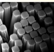
With the proper design of size, shape, and pattern of the carbon nanotubes, it has been further discovered that these synthetic gecko tapes can also be self-cleaning. Reversible adhesion and the self-cleaning effect can be demonstrated through either rinsing with water, or by mechanical cleaning of the surface. The results show that the shear stress of the cleaned samples are 60-90% of those for the pristine, unsoiled samples.
